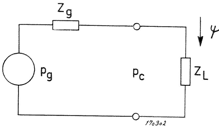
Fig.2.17. Equivalent circuit for the orifice of the Voice Type 4219
