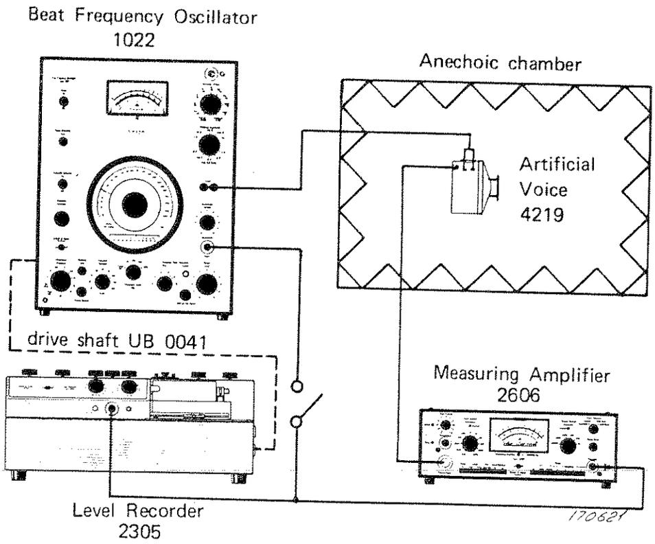
Fig.2.3. Measuring arrangement used for recording the free field characteristics of the Artificial Voice, measured at the orifice
