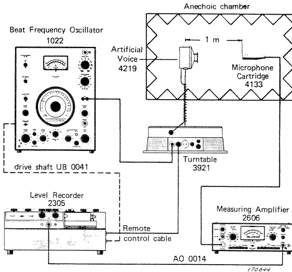
Fig.2.15. Measuring arrangement for recording the angular variation of sound pressure at a distance of 1 meter from the Voice
