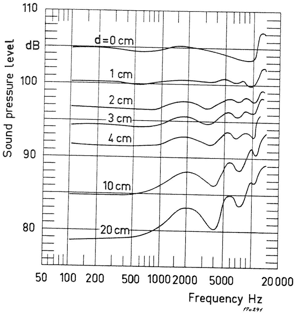
Fig.2.6. The variation of sound pressure with frequency and distance using the arrangement shown in Fig.2.5.
