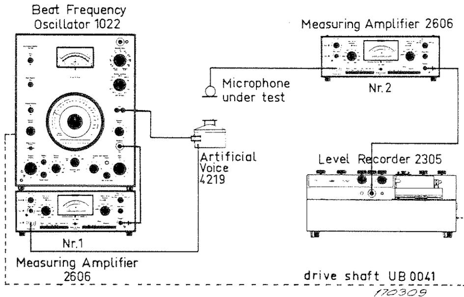
*Fig.3.1. Measuring arrangement for recording the frequency response of a microphone*
