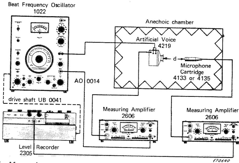
Fig.2.5. Measuring arrangement used for recording the free field characteristics of the Artificial Voice
