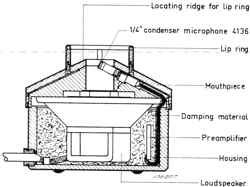
*Fig.2.2. Sectional view of the Artificial Voice Type 4219*
