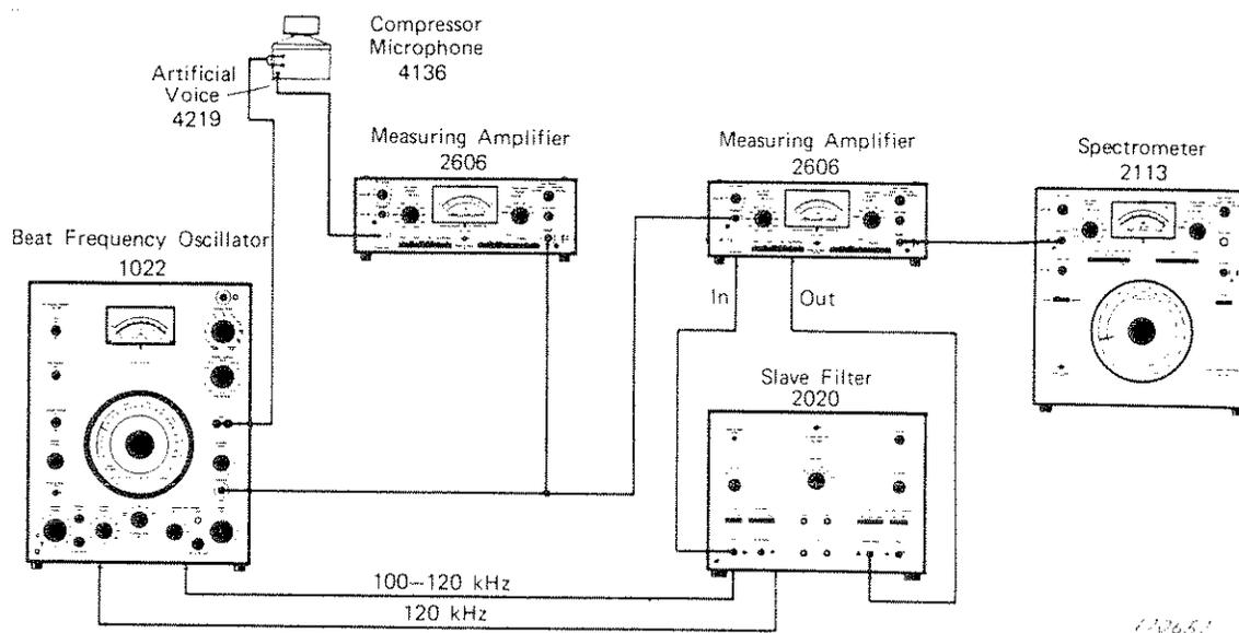
Fig.2.13. Measuring arrangement for recording the frequency characteristics, and the harmonic components produced by the Artificial Voice Type 4219 for a closed mouth opening
