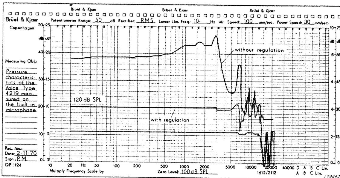
Fig.2.12. Pressure characteristics of the Artificial Voice for a closed mouth opening
