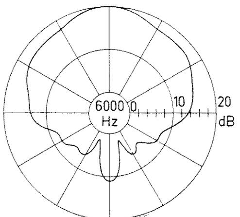
Fig.2.16. Angular variation of sound pressure at a distance of 1 meter from the Voice
