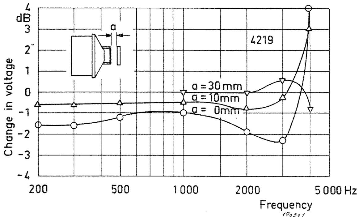
Fig.2.18. Change of voltage across the loudspeaker of the Type 4219 Artificial Voice when an obstacle is presented before the orifice
