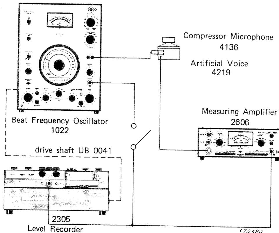
Fig.2.11. Measuring arrangement used for recording the pressure characteristic of the Artificial Voice for a closed mouth opening
